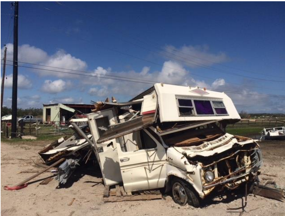
Photo: One of many RVs that were destroyed by hurricane wind forces and airborne debris.
